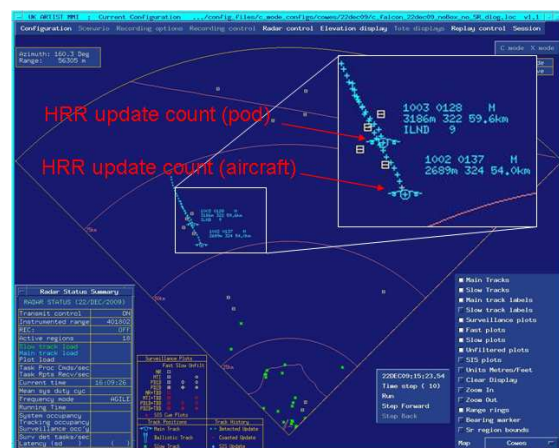
Figure 14 – PPI display from high range resolution (HRR) trial
